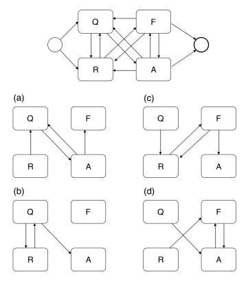
Figure 3.3: The QRFA model for conversational search composed of the "four virtuous cycles of information-seeking": (a) question answering loop, (b) query refinement loop, (c) offer refinement loop, (d) answer refinement loop.
