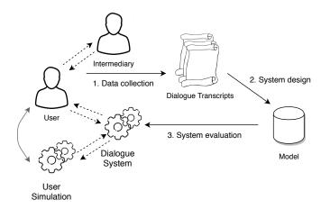
Figure 6.2: End-to-end methodology for designing a dialogue system.
